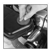
Turn the Suds Control Valve to the OFF position. Go back over the floor to thoroughly clean the floor and to pick up excess solution.
