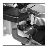
Taking care to avoid spilling liquid on the unit or the floor, place the opening in the bottom of the Shampoo Tank over the Air Exhaust Port.
