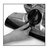
2 Turn the Belt Lifter counterclockwise until the red arrows line up to convert the unit to a straight suction cleaner.
