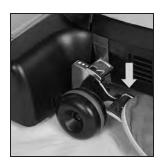
5 Press the Toe Touch Control Upper Pedal repeatedly until the Tile and Grout brush roll contacts the floor. Move the cleaner over the area to be cleaned. Spray additional cleaner as needed.
