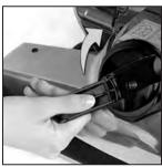
Turn the Belt Lifter clockwise until the green arrows line up.
