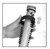
Slide off the old belt and replace with a new one.
