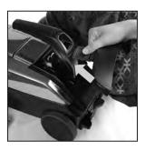
A Bend the Outer Permanent Bag in half and insert the Bag Latch Tab into the slot on the Portable Handle, with zipper facing up.
