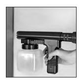
Squeeze the trigger fully and use slow, sweeping motions when spraying.
