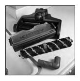
Disassemble and clean all parts of the Multi-Surface Shampoo System using a mixture of 50% ammonia and 50% water to remove any build up of Kirby® Miracle Shine. Allow parts to dry before storage. If necessary, wipe off bottom of the Kirby® system with soft rag dampened with a mixture of 50% ammonia and 50% water
