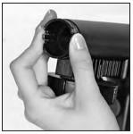
3 Press the two latches on the front of the nozzle jet, pull it out, and thoroughly rinse. Fill the jar with water, reattach and spray water until clear.
