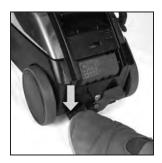
$2^{\,\rm Put}\, {\sf Tech}\, {\sf Drive}^{\otimes}\, {\sf power}\, {\sf assist}$  in neutral by pushing the left "N" neutral pedal down.
