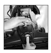
6 Turn the Accessory Lock counterclockwise. Lift off the Multi-Surface Shampoo System and carry it to the sink.
