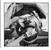
${\bf 5}$  Raise the Headlight Hood. Turn the Belt Lifter counterclock wise until the red arrows line up.
