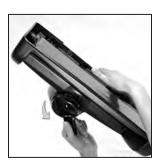
Turn the Multi-Surface Shampoo System over. While pushing up on the belt with your finger, use the handle on the Belt Lifter to turn it counterclockwise until the red arrows line up. The Belt Lifter Hook will catch and stretch the belt.
