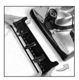
Turn the unit off. Step on the bottom pedal of the Toe-Touch Control to raise the Power Nozzle. Slide the Hard Floor Pad under the nozzle and press up until the clips lock in place.
