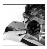
8 Flip out the handle on the Belt Lifter and use it to turn the Belt Lifter clockwise until the green arrows line up. This will engage the belt so the Brush Roll will spin. See page 17. Lower the Headlight Hood.
