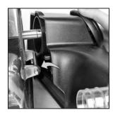
Connect the hooks on the rear of the Multi-Surface Shampoo System to the Attaching Bar.
