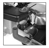
17 Taking care to avoid spilling liquid on the unit or the floor, place the opening in the bottom of the Shampoo Tank over the Air Exhaust Port.
