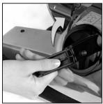
**Q** Turn the Belt Lifter clockwise until the green arrows line up.
