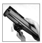
Turn the Multi-Surface Shampoo System over. While pushing up on the belt with your finger, use the handle on the Belt Lifter to turn it counterclockwise until the red arrows line up. The Belt Lifter Hook will catch and stretch the belt.
