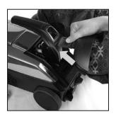
$m{4}$  Bend the Outer Permanent Bag in half and insert the Bag Latch Tab into the slot on the Portable Handle, with zipper facing up.
