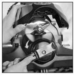
$5\,\text{Raise}$  the Headlight Hood. Turn the Belt Lifter counterclockwise until the red arrows line up.
