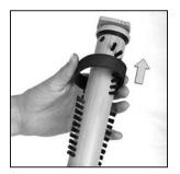
Slide off the old belt and replace with a new one.
