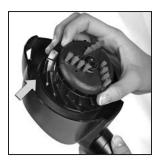
2 Lift the turbine out of the tool and remove any particles or lint from the turbine and tool cavity.
