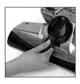
Raise the Headlight Hood. Flip out the handle on the Belt Lifter.
