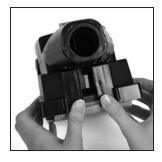
With the Turbo Accessory on a level surface, reattach the sander dust shroud with the opening to the rear. Insert the Attachment Hose.
