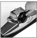
Turn the Belt Lifter counterclockwise until the red arrows line up. The belt should catch on the hook inside the nozzle. Reattach the Power Nozzle to the unit.
