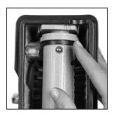
2 Rotate the Brush Roll ends to the desired setting: 1, 2 or 3 notches. Make sure the setting is the same on both ends. The greater the number of notches, the further the bristles are extended.
