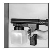
Squeeze the trigger fully and use slow, sweeping motions 3 when spraying.
