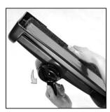
While pushing up on the belt with your finger, use the handle on the Belt Lifter to turn it counterclockwise until the red arrows line up. The Belt Lifter Hook will catch and stretch the belt.
