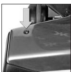
Turn the unit on and check that the Brush Roll Indicator Light is on. This means that the brush roll is spinning.
