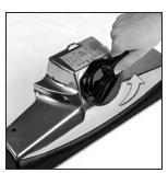
5 Flip out the handle on the Belt Lifter on the Power Nozzle. Turn it counterclockwise until the red arrows line up. The hook should catch and stretch the Belt inside the Power Nozzle.
