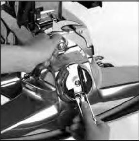
**4** Turn the Accessory Lock counterclockwise to release the Power Nozzle. Lift the Power Nozzle away. Clean any lint, hair or debris from the Motor Shaft.
