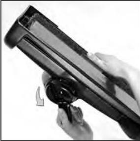
7 While pushing up on the belt with your finger, use the handle on the Belt Lifter to turn it counterclockwise until the red arrows line up. The Belt Lifter Hook will catch and stretch the belt.
