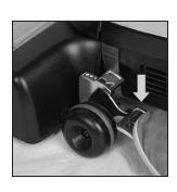
Press the Toe Touch Control Upper Pedal repeatedly until the Rotary Mop contacts the floor. Move the cleaner over the area to be cleaned. Spray additional cleaner as needed.
