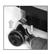
Press the Toe-Touch Control Bottom Pedal all the way down to raise the front of the unit.
