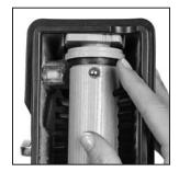
2 Rotate the Brush Roll ends to the desired setting: 1, 2 or 3 notches. Make sure the setting is the same on both ends. The greater the number of notches, the further the bristles are extended.
