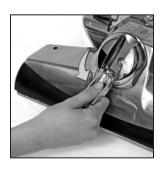
Raise the Headlight Hood. Flip out the handle on the Belt Lifter. Use it to turn the Belt Lifter counterclockwise until the red arrows line up.
