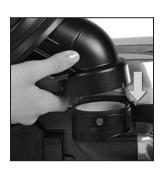
With the arrows lined up, slide the Mini Em-Tor® collector on to the Air Exhaust Port. Rotate it toward the unit to lock in place.
