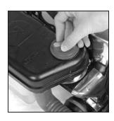
6 Turn the Suds Control Valve clockwise to the Hard Floor Setting. Put Tech Drive® power assist in neutral. Turn the unit on. As the unit is moved back and forth, cleaning solution will release and the Rotary Mop will scrub the floor.
