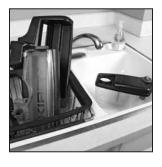
At the sink, discard any remaining liquid in the Shampoo Tank. Remove and clean the Suds Screen Cap, tank cap and sponge filter. Rinse out the Shampoo Tank with cold water and replace the Suds Screen Cap, tank cap and sponge filter. Allow all parts to dry thoroughly before reassembling.
