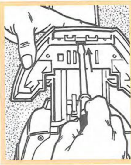
LIGHT BULB REPLACEMENT
