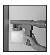
3 Use slow, sweeping motions to spray the desired area with solution. Always squeeze the trigger fully to permit maximum flow. This will give you the best spray control. □
