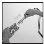
With the wax roller bag facing the hooked end of the long roller handle, push the wax roller over the connector on the bottom of the handle until secure.
