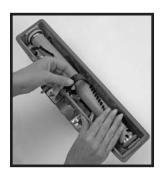
Make sure the Brush Roll Bristle Height Adjustment setting (1, 2, or 3) is the same on both ends as when the brush was removed. See below for discussion of the Brush Roll Bristle Height Adjustment (1, 2, or 3). Place the belt and Brush Roll back into the nozzle. One of the plastic Brush Roll ends is larger than the other, thus the Brush Roll will only fit in the nozzle one way.
