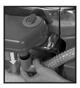
Turn the Suds Control Valve fully to the left (counter-clockwise) to the OFF position.
