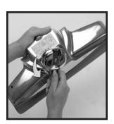
Using the handle on the Belt Lifter ②, turn it to the left (counterclockwise) until the red arrows line up. This will stretch the belt in preparation for returning the nozzle to the *Sentria*® system.
