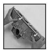
Replace the Rug Plate by placing it on the front of the bumper first and then pulling it over the bumper on the rear of the Power Nozzle . Secure the Rug Plate using the two latches that hold it in place.
