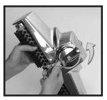
While holding the belt in place, use the handle on the Belt Lifter to turn it left (counter-clockwise) until the red arrows line up. The Belt Lifter hook will catch the belt and stretch it upward into the nozzle.
