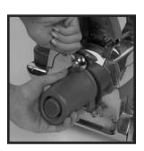
When using the blower attachments, the Air Intake Guard must be attached to the front of the unit.
