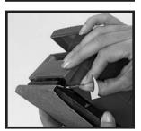
3 Select the correct grade of sandpaper needed for the job. Use fine paper for a smooth finish and coarse paper to clear rough surfaces or remove paint.
