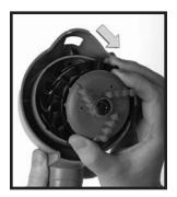
2 Lift the center Brush/Air Turbine out of the tool and remove any particles or lint from the brush and turbine. Also remove any particles left in the tool cavity. ▶
