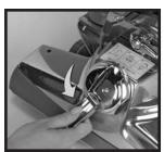
2 Flip out the handle on the Belt Lifter ②. Use it to turn the Belt Lifter fully to the left (counter-clockwise) until it stops and the red arrows line up. This stretches the belt and lifts it off the motor shaft. Return the handle on the Belt Lifter to its closed position.
