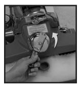
Raise the Headlight Hood ②. Release the belt by turning the Belt Lifter to the left (counter-clockwise) until the red arrows line up.
