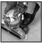
3 Lower the Carpet Fluffer Nozzle one notch at a time by pushing the Toe-Touch Control Upper Pedal ⑧. The instant the brush contacts the carpet, stop lowering the brush. ➤
