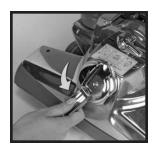
Flip out the handle on the Belt Lifter ②. Use it to turn the Belt Lifter all the way to the left (counter-clockwise) until the red arrows line up (see page 9). Return the handle on the Belt Lifter to its closed position.
