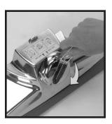
Release the belt tension by using the handle on the Belt Lifter to turn it all the way to the right (clockwise) until the green arrows line up.
