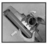
While pushing up on the belt with your finger, use the handle on the Belt Lifter to turn it left (counter-clockwise looking at it from the front) until the red arrows line up. (The Belt Lifter Hook will catch and stretch the belt.)
