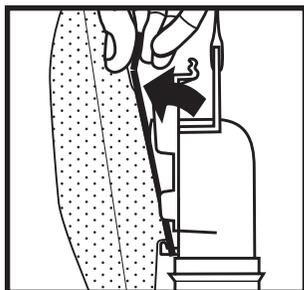
**To remove a used Disposable Filter Bag.**
